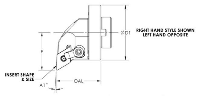
EXAMPLE: HEAD WITH "H32" ( $\emptyset$ 2.0") BAR COUPLING ( $\emptyset$ D1), RIGHT HAND, DNMG-432 INSERT @ -3° LEAD ANGLE (A1°) AND COOLANT SUPPLY.
