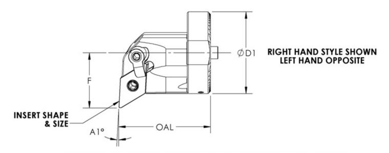
EXAMPLE: HEAD WITH Ø40MM BAR COUPLING (ØD1), RIGHT HAND, DNMG-432 INSERT @ -3° LEAD ANGLE (A1°) AND COOLANT SUPPLY.
